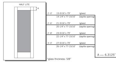
A — distance from top of door to top of cut-out
